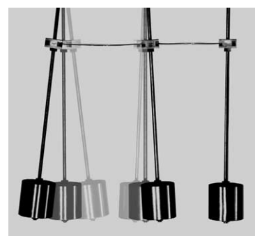
Fig. 3. Experimental pendulum system used to demonstrate the correspondence between TOCSY transfer in isotropic mixing experiments and the transfer of energy between coupled pendulums. Each pendulum has a weight of about 6 kg. The couplings between the pendulums are provided by U-shaped steel springs.
